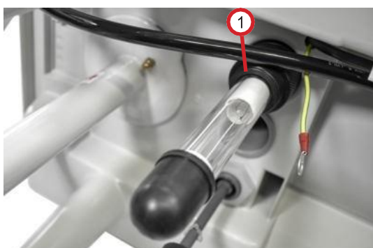
Abb. 8.1.2.6: UV-Lampe in Quarzglasröhre.
