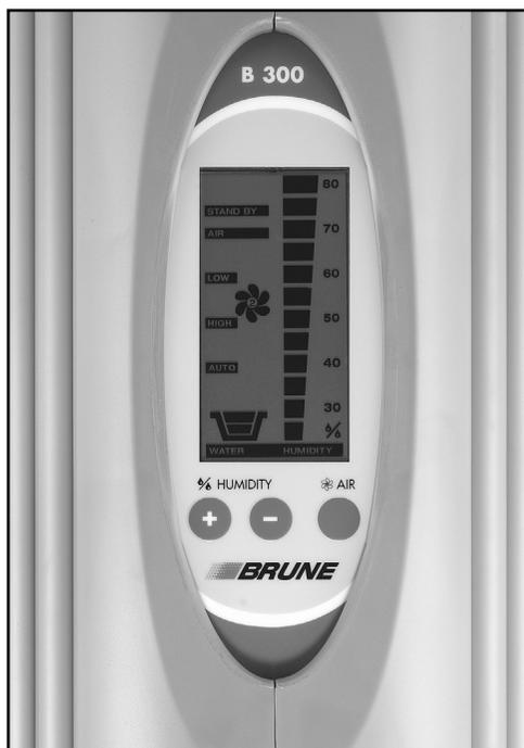
The indicator display and setting of the relative humidity takes place in 5% increments. Therefore, the values may deviate when using other control devices. At 3% and 8%, the display jumps over to the next higher value (e.g. actual humidity = 43% corresponds to =45%)
