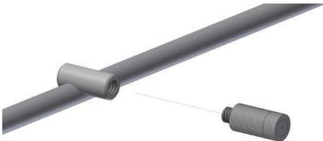
Fig. 20: Insertion des buses
