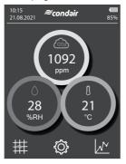
6. Check the CO<sub>2</sub> value. If it is within the range of 400 +/-25 ppm, the calibration was successful. If the value is above or below this, repeat the calibration.
