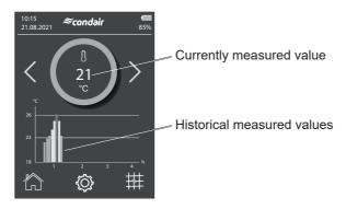
This view shows the course of the measured room temperature over a maximum of 4 hours.
