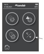
Switch between degrees Celsius / degrees Fahrenheit by pressing the icon. The set value is displayed in the lower gray box with °C or °F.
