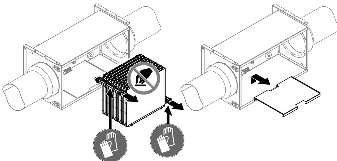
*Fig. 21: Removing the humidifier insert and base panel*
