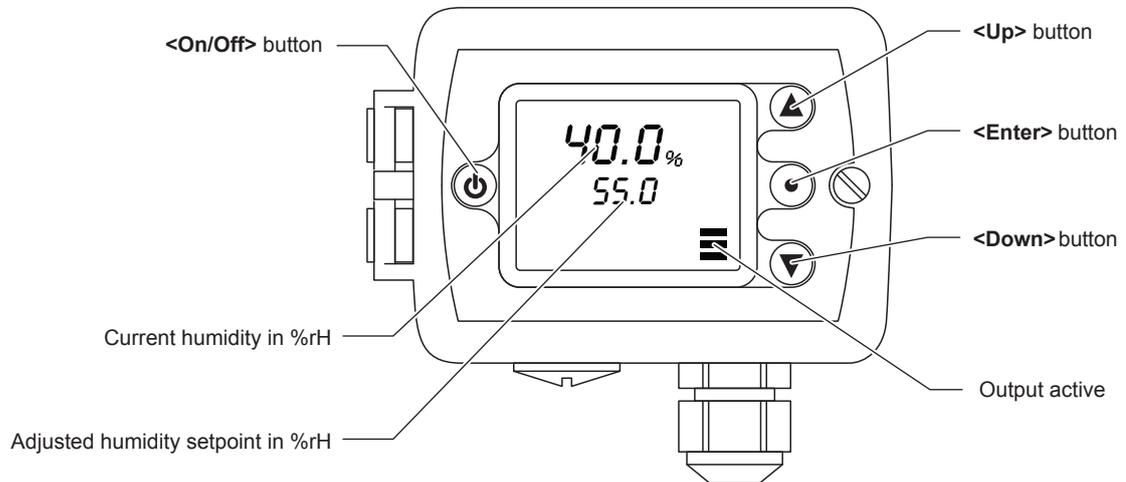
Fig. 10: Maximum humidistat operating elements
