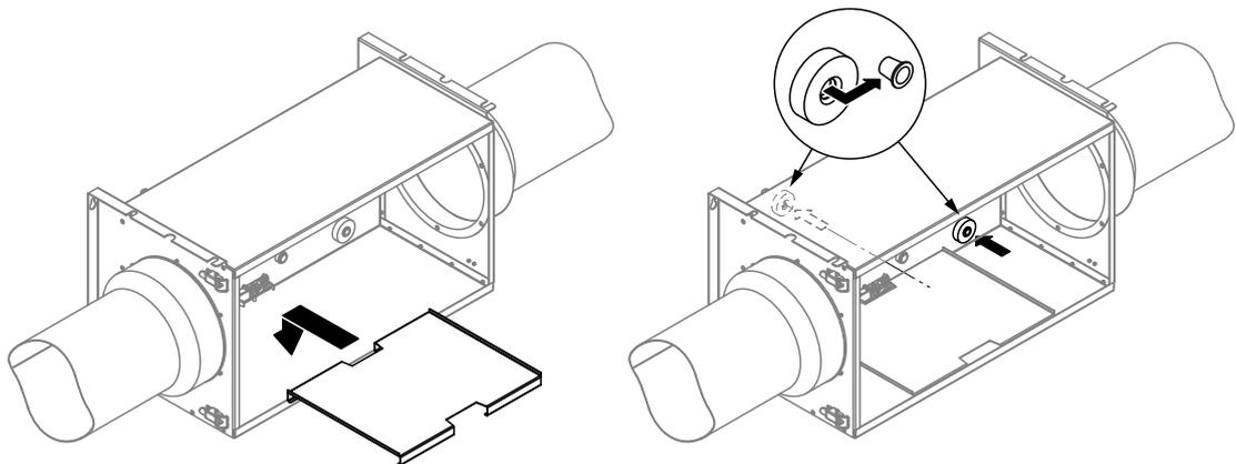
*Fig. 6: Insert the base panel and remove the sealing plugs*
