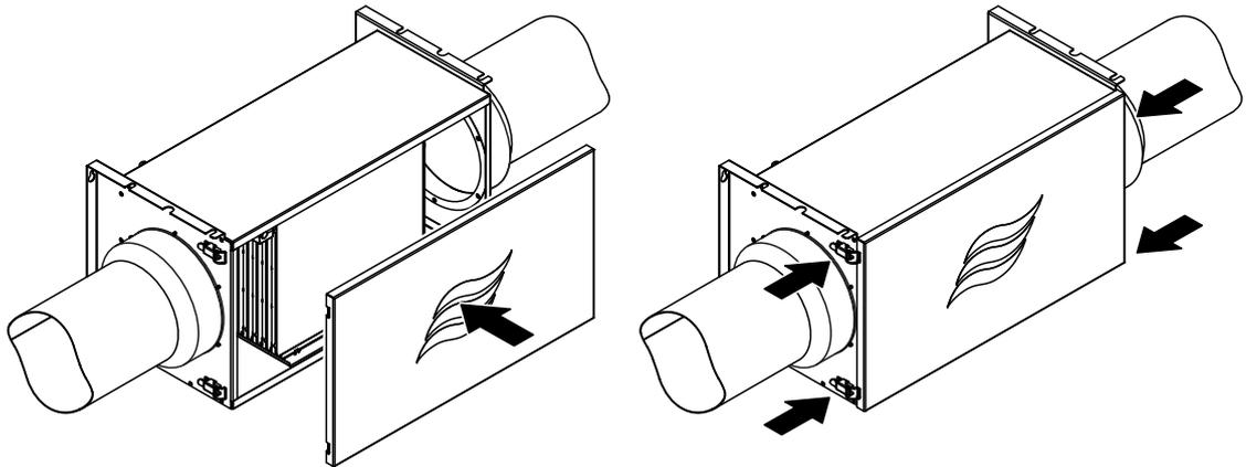
*Fig. 25: Closing the humidifier unit*
