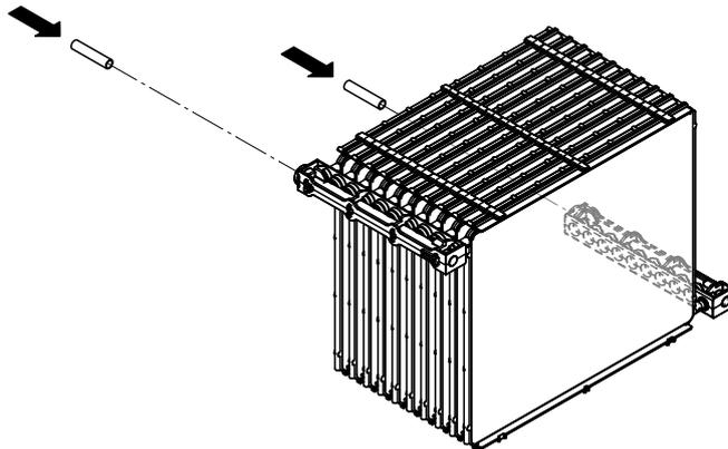
*Fig. 7: Insert the hose sections into the plug connectors*
