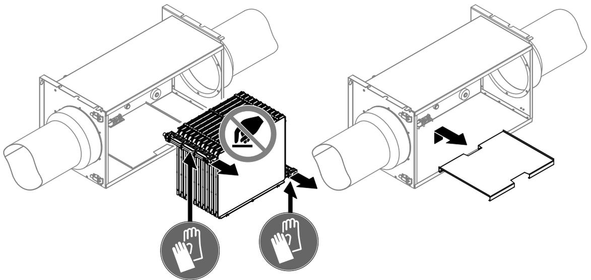
*Fig. 15: Removing the humidifier insert and base panel*
