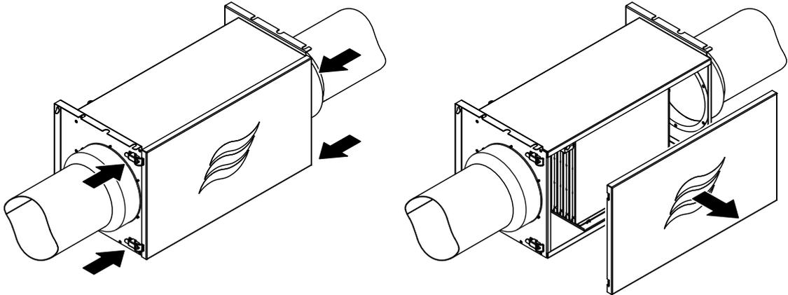
Fig. 14: Opening the humidifier unit
